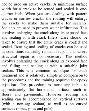
Routing and sealing is used to treat both fine pattern cracks and larger, isolated cracks. A common and effective use is for waterproofing by sealing cracks on the concrete surface where water stands, or where hydrostatic pressure is applied. This treatment reduces the ability of moisture to reach the reinforcing steel or pass through the concrete, causing surface stains or other problems.
